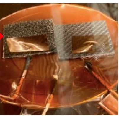
Flax fiber took less time to heat up to 170°C and less time to cool down to 50°C compared to glass fiber
