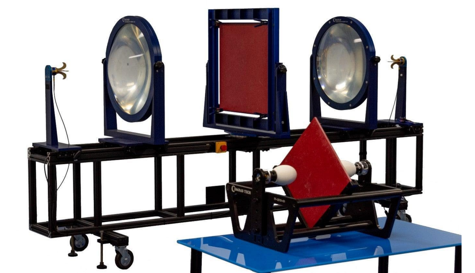
Compass Microwave Focused Beam System Source: Compass Technology Group
