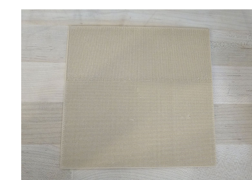
Logpile printed pattern 150mm x 150mm x 1.7mm
