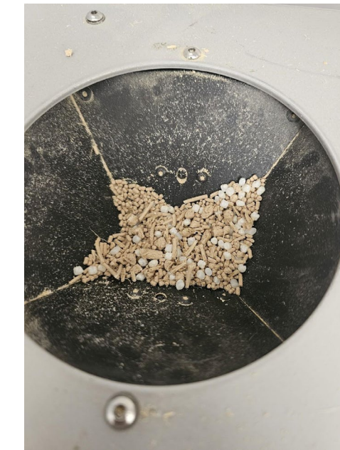
Strontium Titanate filled ABS pellets loaded into the 3Devo Next. Source: Luke Ballenger
