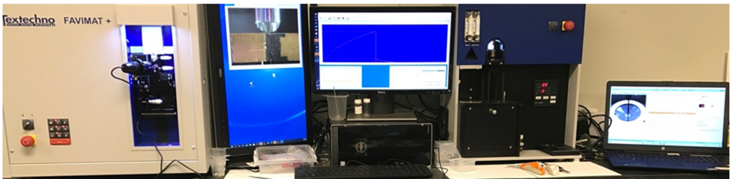
Single fiber pullout specimen preparation and testing
