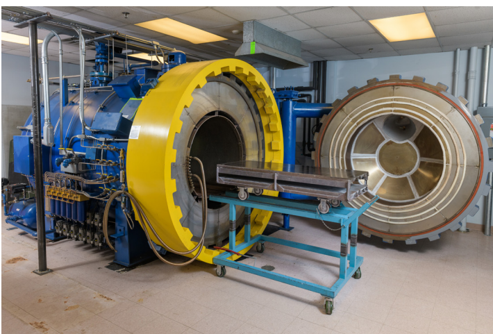
TEC – 1000°F, 515 psi Processing Autoclave
