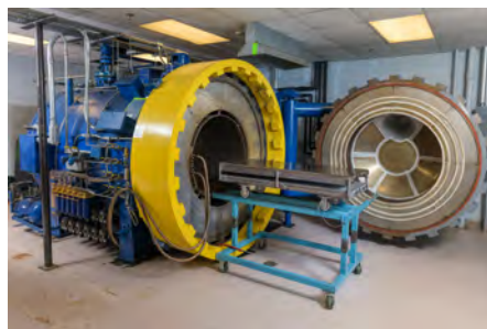
TEC – 1000°F, 515 psi Processing Autoclave
