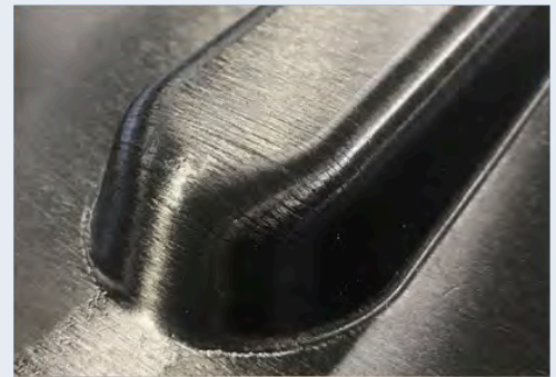
250gsm quasi-isotropic [0/90/45/-45] s laminate
