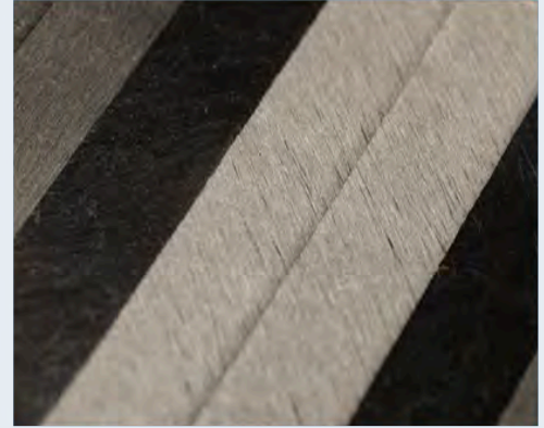
250gsm quasi-isotropic [0/90/45/-45] s laminate
