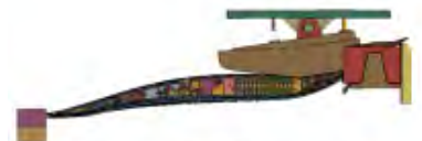
Composite B-Pillar Crash Modeling with LS-Dyna
