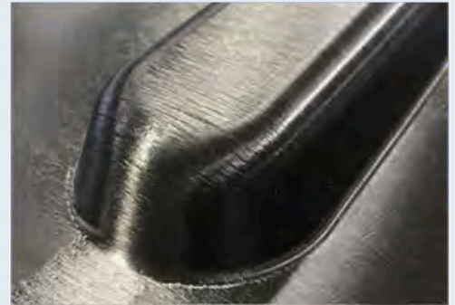
250gsm quasi-isotropic [0/90/45/-45]s laminate
