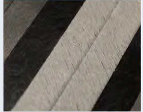
250gsm quasi-isotropic [0/90/45/-45]s laminate
