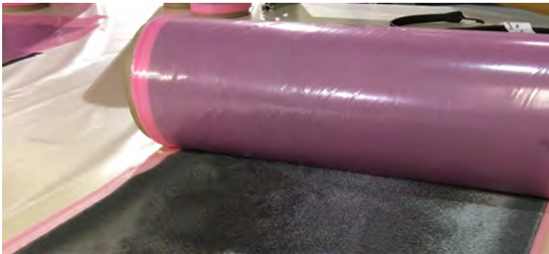
Continuous TuFF sheet of Highly Aligned Short Fiber
