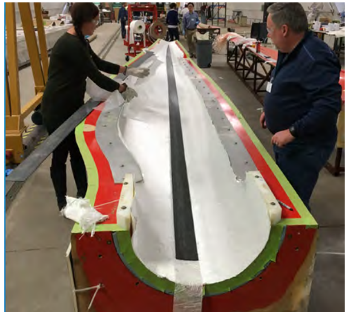
UD-CCM is developing a sustainable, low-cost material and process solution for recycled spar caps for offshore wind blades, reducing embodied energy by 80% and fiber material cost by 70%
