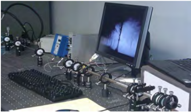
High strain rate dynamic microdroplet test
